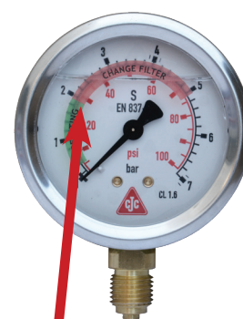
CJC™ Pressure Gauge WITH the sticker indicating when to change the CJC™ Filter Insert
